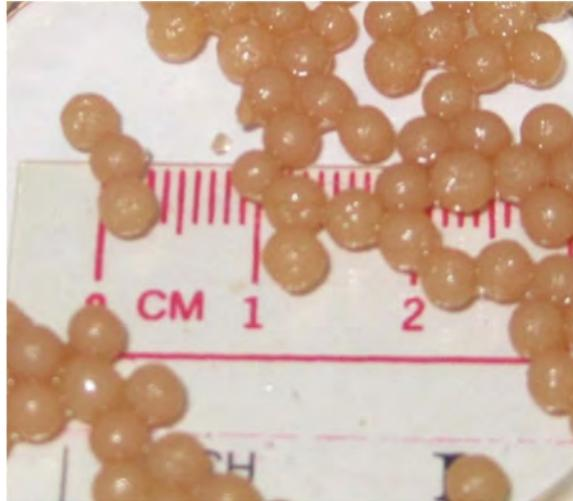
**Figure 1.** Image of the synthesized metal-cross-linked alginate (MCA) beads
