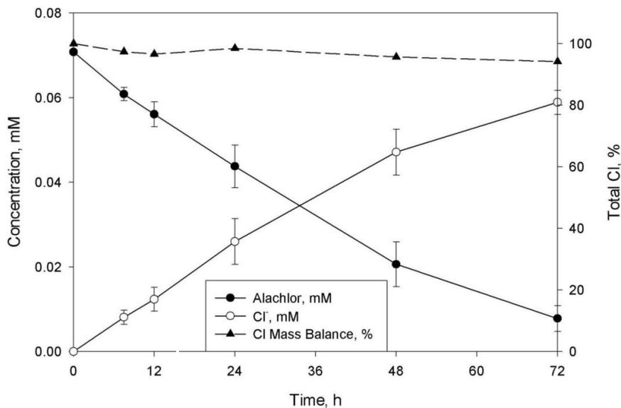
**Figure 6.** Chloride mass balance for alachlor degradation by nZVI. Chloride mass balance ranged from 94% to 98%. The vertical error bars indicate  $\pm$  standard deviations. Data points are joined by straight lines for ease of reading only and do not represent trends.
