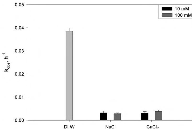
**Figure 7.** Comparison of observed alachlor degradation reaction rate constant under different ionic strength conditions. “DI W” stands for “deionized water”; trial has ionic strength of zero. Error bars represent 95% CI.
