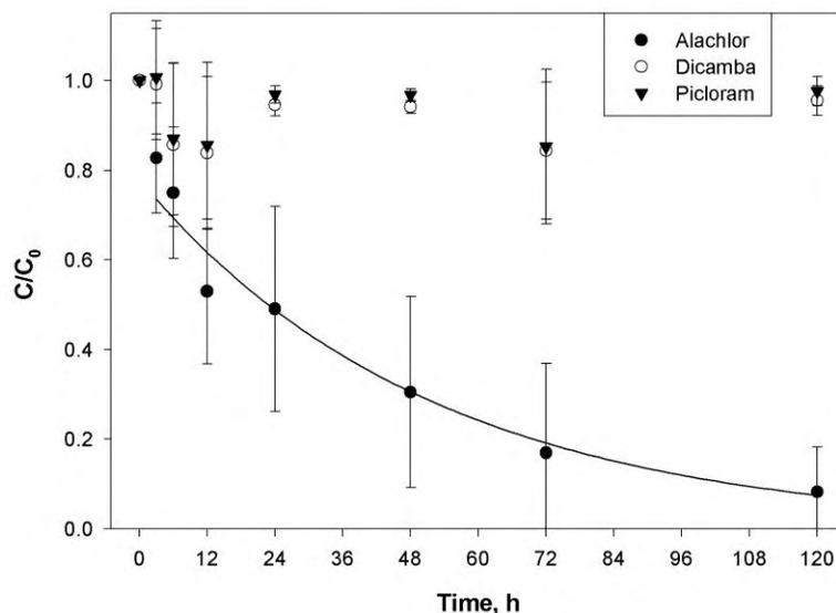
**Figure 8.** Reduction of alachlor in alginate-nZVI system. First data point is not considered in the model to account for initial diffusion into the alginate beads. The vertical error bars indicate  $\pm$  standard deviations.
