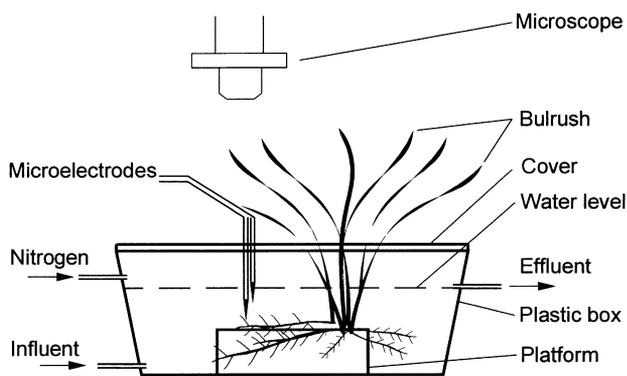
**Figure 1.** Schematic of the reactor used for active root count. A 3D micromanipulator was used for microelectrode movement. The headspace above the wastewater was streamed with nitrogen gas to prevent diffusional oxygen transfer. A critical evaluation of the reactor design and its possible impact on results are presented in the discussion part of this article.
