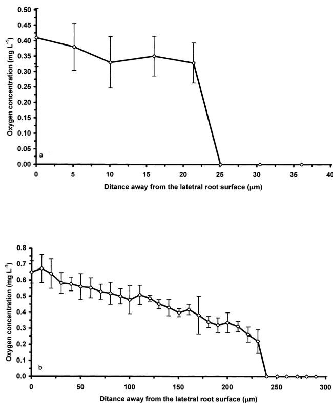
**Figure 3.** DO microprofiles of (a) a brown lateral and (b) a white lateral as the microelectrode was moved away from the root surface in the radial direction. Error bars representing  $\pm 1$  standard deviation (*SD*) were calculated from five consecutive stable readings. All measurements were done inside the Faraday cage and in the reactor shown in Figure 1.
