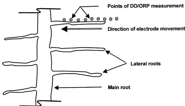
**Figure 2.** Schematic of a section of a main root with the laterals. The microelectrode (DO or ORP) was first manually positioned at or near the tip of the lateral root and then moved in steps of  $5, 10, 50,$  or  $250 \mu\text{m}$  towards the body of the main root.
